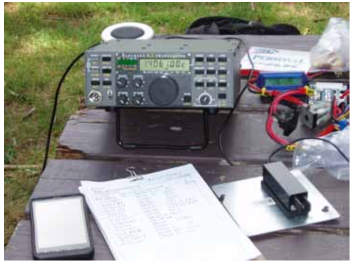
N1FJ's typical SOTA setup on Mt. Grace in Warwick, Mass. Log shows several dx contacts with Great Britain and France, along with many stateside SOTA chasers, including WN1E & KK1W. Operation was 20 meter CW, 5 or 10 watts to a dipole strung from the fire tower to a tree.
