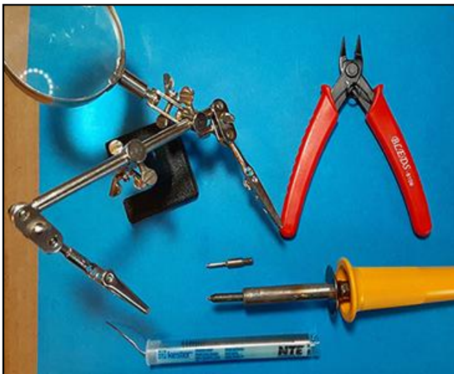
(photo 2) Useful tools for kit building: "Hand Free" Holder, Wire Cutters, Solder, and small tip for soldering Iron
