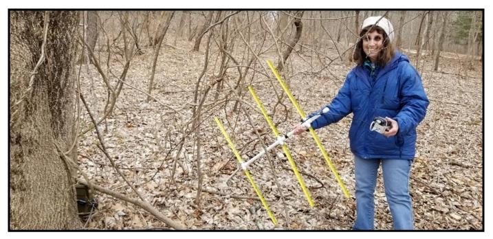
Above is a picture of Faye with the antenna and radio and attenuator pointing right at the foxbox.
