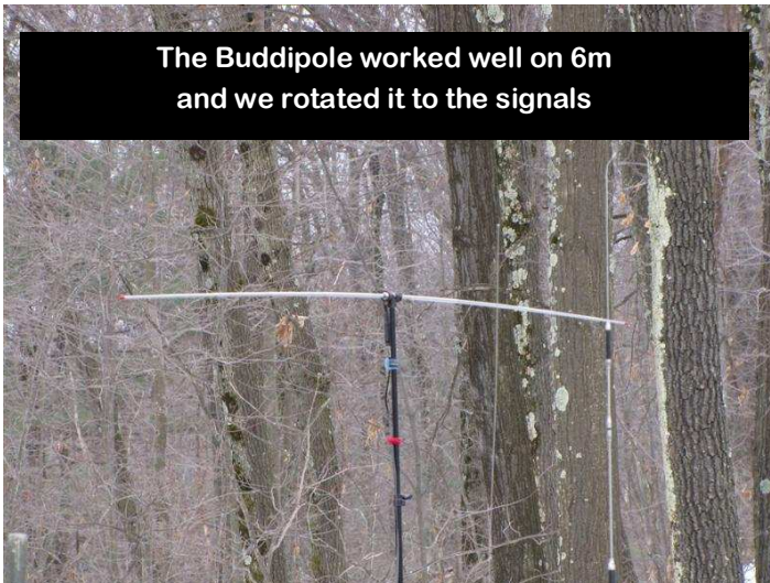
The Buddipole on the right is on a 8 foot collapsible pole and tripod. It all breaks down to a bag that's about 30 inches wide by 4 inches deep! Visit www.buddipole.com for more info
