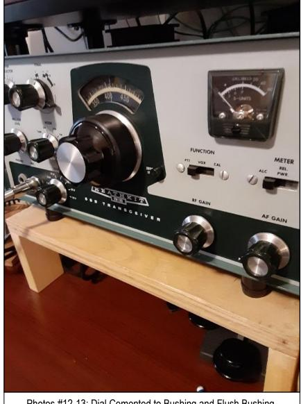
Photos #12-13: Dial Cemented to Bushing and Flush Bushing. (Photo Credit: B.Cook)
