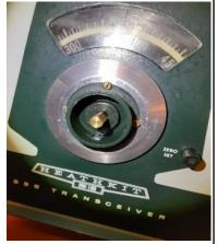
Photos 5 and 6, Mounting Tabs on Vernier Dial and VFO Shaft and Opening (Photo Credit: Cook)
