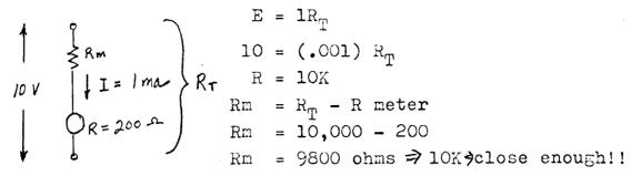
By using ohm's law  $R_{\rm T}$  = 10K. The internal meter resistance of 200 ohms can be disregarded since this is much smaller than the 10K calculated to draw 1 ma from a 10 volt source. Therefore, a 10K series resistor is all that is necessay to make a 0-10V voltmeter.
