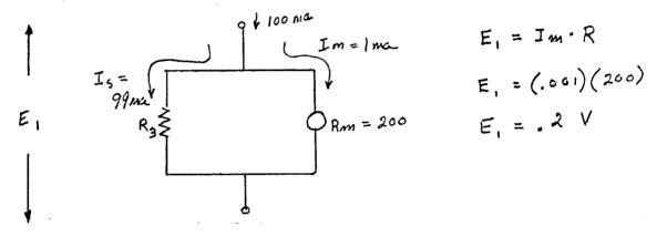
First calculate the voltage drop across your basic meter. This happens to be .2 V for our example. Notice most of the current flows through our shunt ( 99ma vs 1 ma through the meter). Using ohm's Law:
