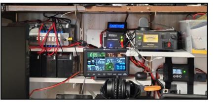
Commercial power powers the 12 VDC power supply that feeds into a West Mountain Radio Epic PWRgate. The PWRgate is also fed by solar panels and SLA batteries. If commercial power fails, the PWRgate switches to batteries fast enough that you don't even notice. The solar panels then take over, recharging the batteries. During normal operations, the power supply maintains the charge on the batteries.
