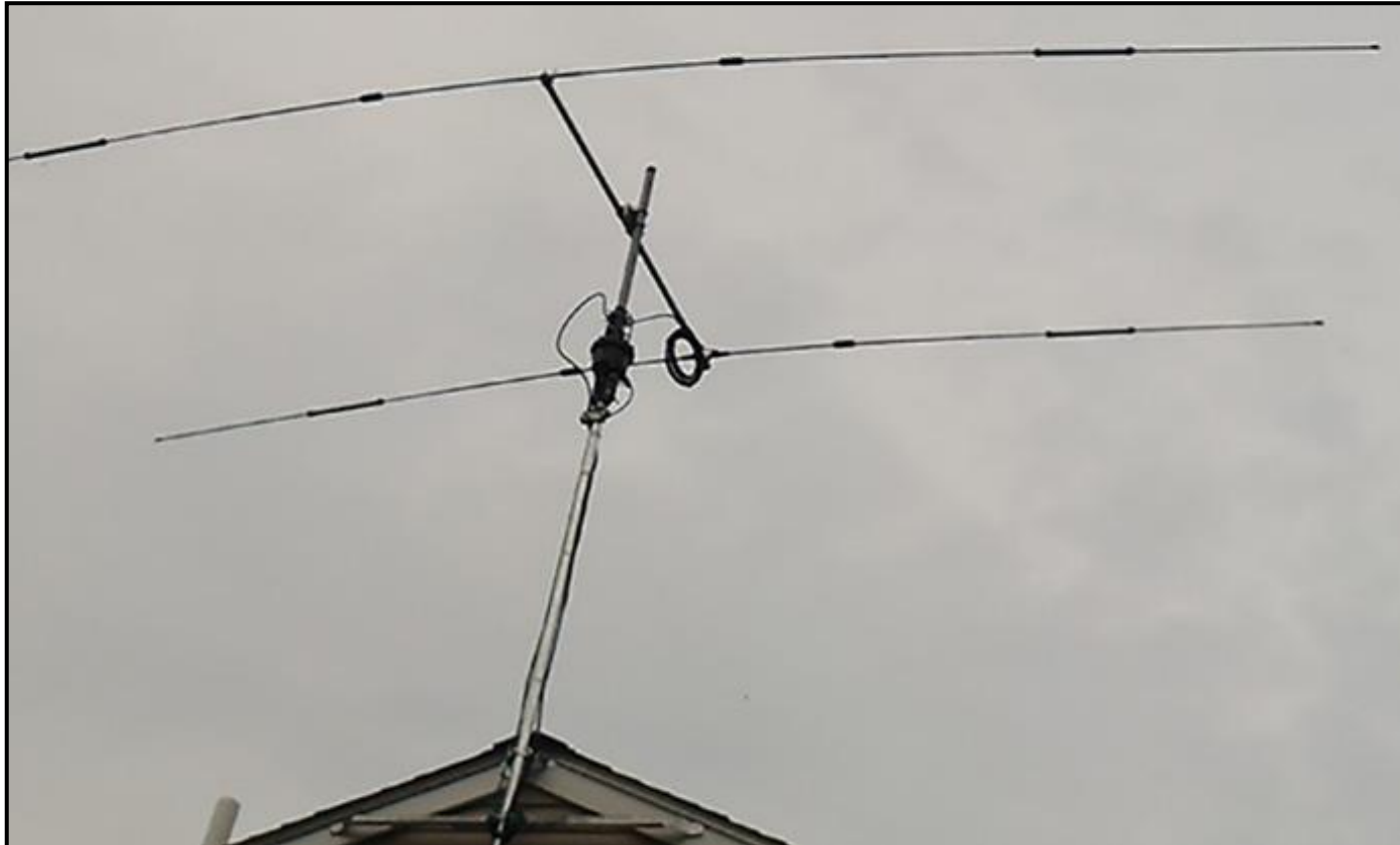
Above: Mosley 2-Element Mini - Yagi Tri-band, 10m, 15m, & 20m Mounted at 30' on a Rohn Mast with a Yaesu Rotor
