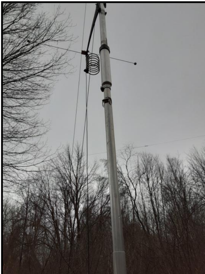
Close-Up of top Bracket with Coil and Tuning Rods for 17M Add-On
