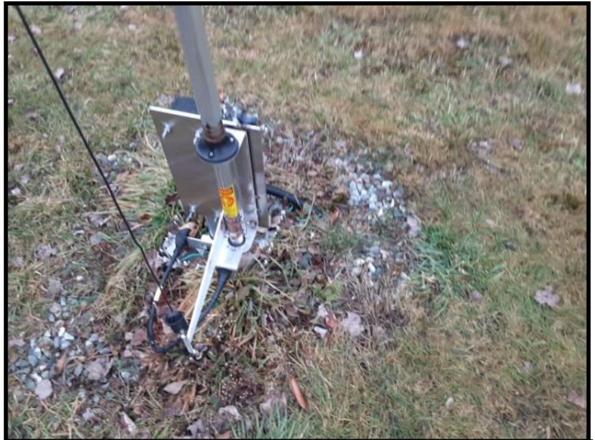
Bottom Bracket and spring-tensioned bracket for Element Wire of 17M Add-On
