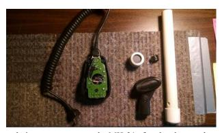
On this second picture, you can see the MH-31 after the electret element was installed.
