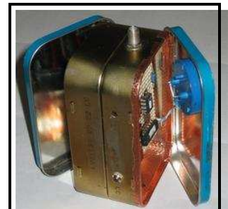
A look at the interior of the shielded side with the copper tape along the edge and inside to eliminate RF interference. All photos by Sam Green, WOPCE.
