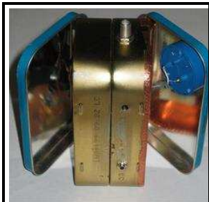
A view of both tins open. Notice the copper tape shielding on the right-hand tin.
