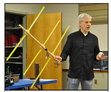
Alan, AB1XB, built a collapsible tape measure RDF yagi antenna. He'll be making a case for it next.
