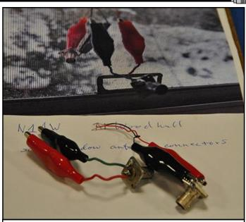
Al passed the wire and alligator clips right through the screen. This won't work with metal screens.
