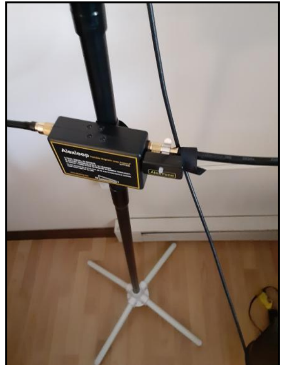
Alexloop on stand with Alextune clipped to PL-259
