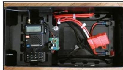
A foxbox is usually an ammo can (metal rectangle can with a battery, radio, interface and antenna locked to a tree or something similar).
