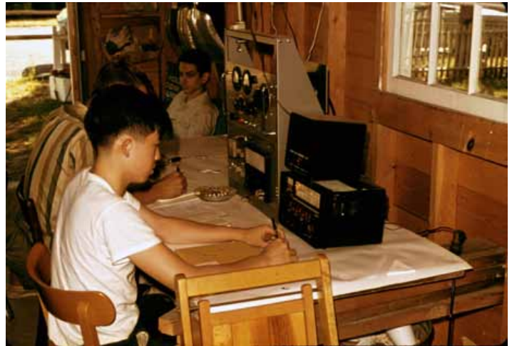
Equipment circa mid 1960's: Drake 2b receiver, Eico 723 60 watt cw transmitter and homebrew vfo mounted in lower rack, homebrew 572B amplifier in upper rack. Note the stack of 2x6's and trash can holding up the operating desk---really roughing it!
