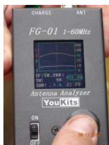
6m swr plot while the antenna was on the ground.
