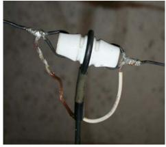
One way to secure your coax feed line is to loop it over the center insulator. Solder all connections using sufficient heat! You may want to protect your solder joints by wrapping them with electrical tape.
