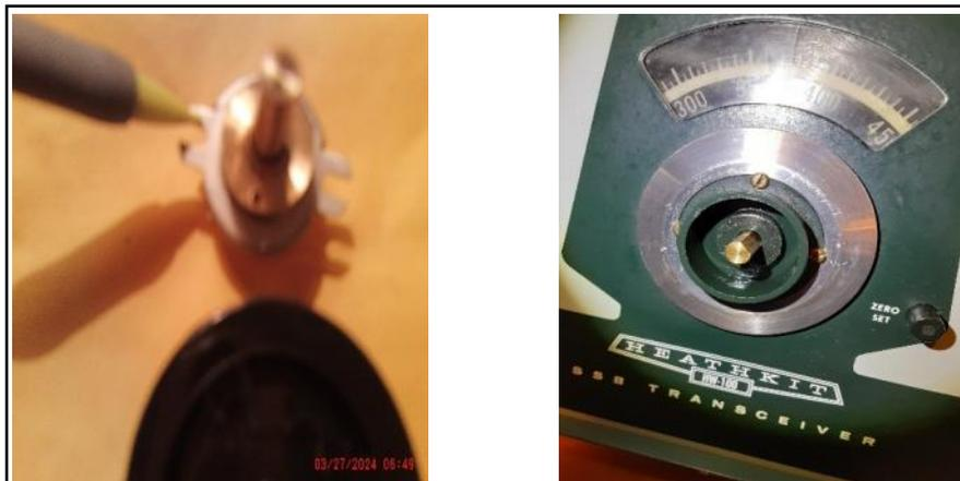
Photos 5 and 6, Mounting Tabs on Vernier Dial and VFO
