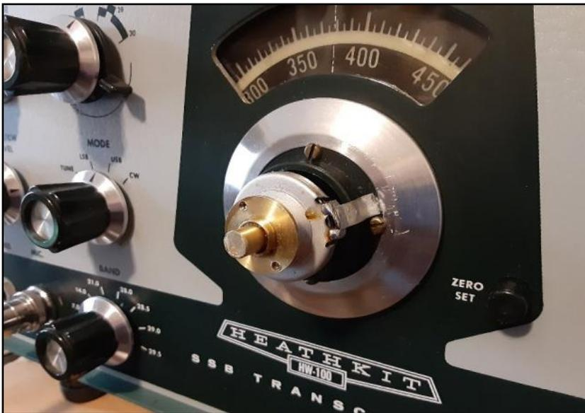
Photo #8: Vernier attached to VFO Variable Capacitor Shaft and Anchored in Place. (Photo Credit: B.Cook)
