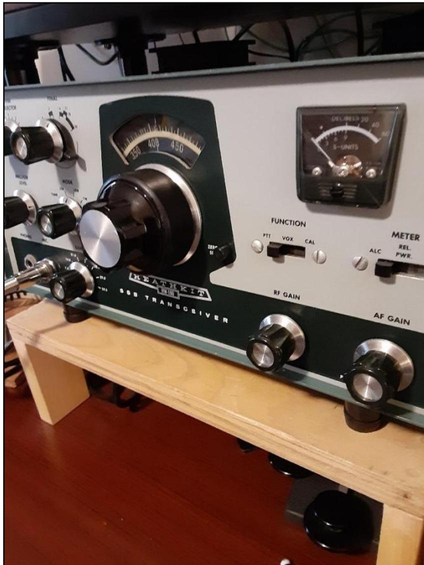
Photos #12-13: Dial Cemented to Bushing and Flush Bushing.
