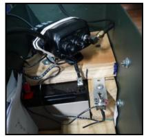
cally places holds the battery in place yet allows removal if needed. We needed a way to keep the HT in place. A bent piece of angle iron does the job nicely. A power switch to turn everything on and off easily. This little switch turns on the radio and interface so everything is off when not in use and not draining the battery. (left)
