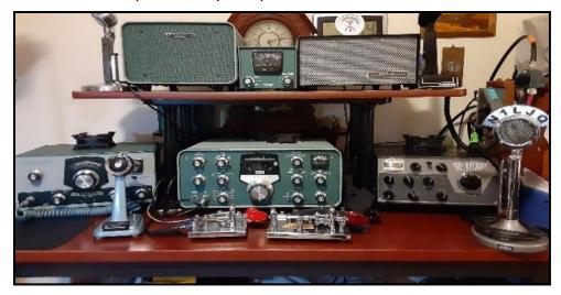
Shown in the photo on the right is a Drake TR-4 Transceiver and above it an MS-4 speaker with a power supply installed – this radio was manufactured in 1965. On the left is a Heathkit SB 101 with a speaker and power supply, as well as an SWR/Power meter above it – all from about 1970. And, of course, there is an Astatic D-104 microphone. Finally, on the left is a Heathkit HW-32A Single Bander for 20 Meters SSB from 1966.
