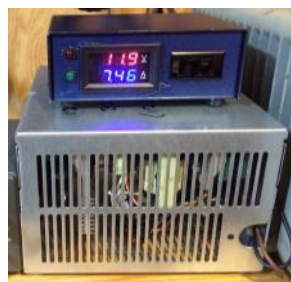
Finished modified PC power supply with monitoring box
