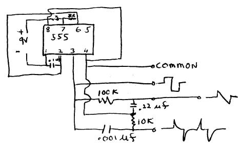
\* is a 7.5K resistor or variable pot \*\* is a 1-3 K resistor or variable pot
