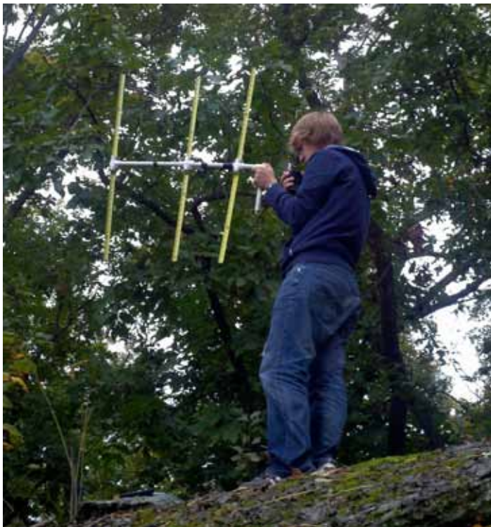
Nick, K1MAZ, shown using a “home built” 2 meter tape measure Yagi on Burley Hill SOTA activation in Connecticut last year.
