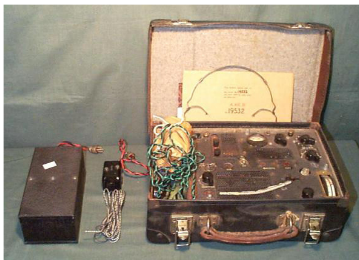
Special Operations Executive, Model Type B, Mark II British suitcase radio.
