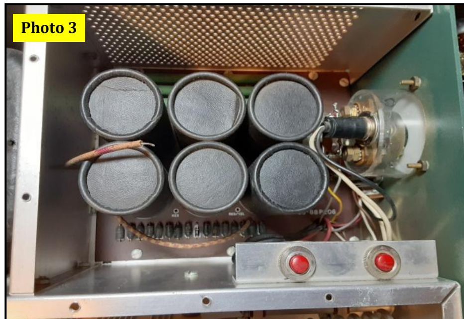
Original Power Supply PCB and Circuit Breakers (Red Buttons) Credit: Harbach.com
