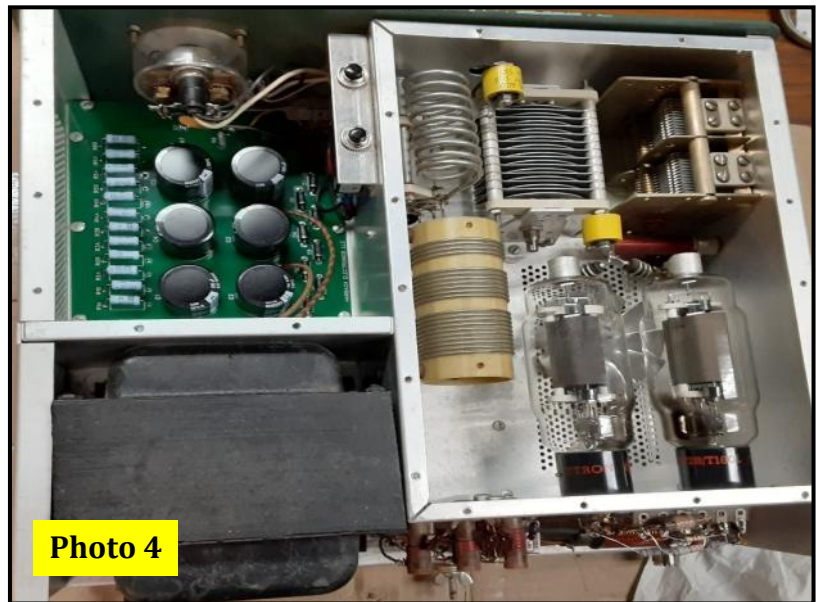
Photo 4 New Power Supply Board and Circuit Breakers Installed Credit: B.Cook
