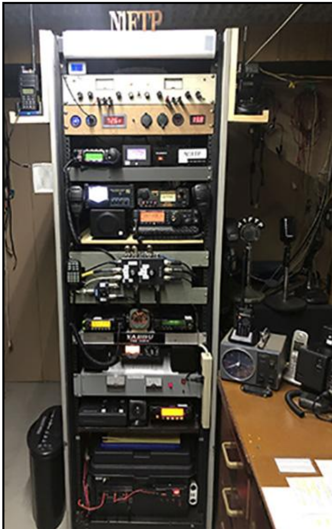
(2) Rack holds VHF/UHF Radio's & Coax Switches
