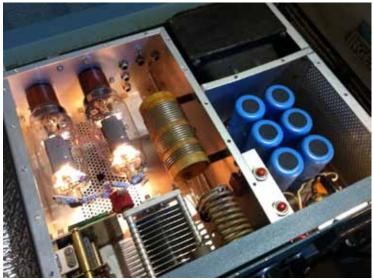
left the amp on for an hour and nothing happened in that time so I decided to put a signal through the amp to see what happens. I went on the 20m band, put the radio into CW and did a tune. I was glad to see around 600W on my watt meter.
