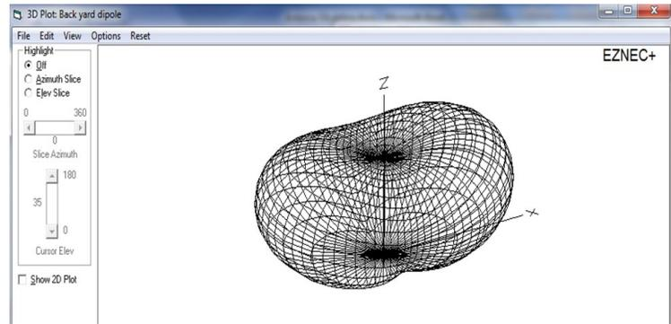
Check the Show 2D Plot. Arrange the windows side by side. Click the Azimuth Slice and change the elevation angle. Notice how the change carries over to the next window.
