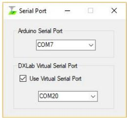
**[Arduino Serial Port]** (Same port as used for loading Arduino software)
