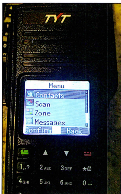
Photo E. The MD-380 HT menu screen. Note that zones is third down on the list.
