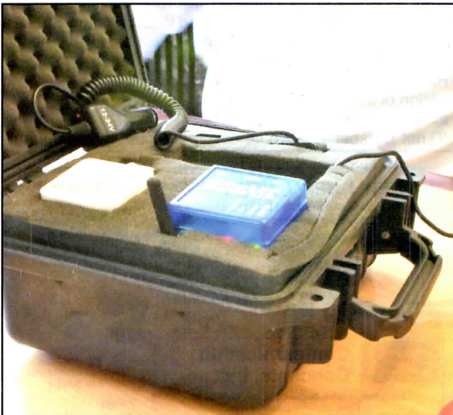
Photo I. W9FE's Shark RF OpenSpot allows Carlos to use DMR on the road or at home with his WiFi connection.
